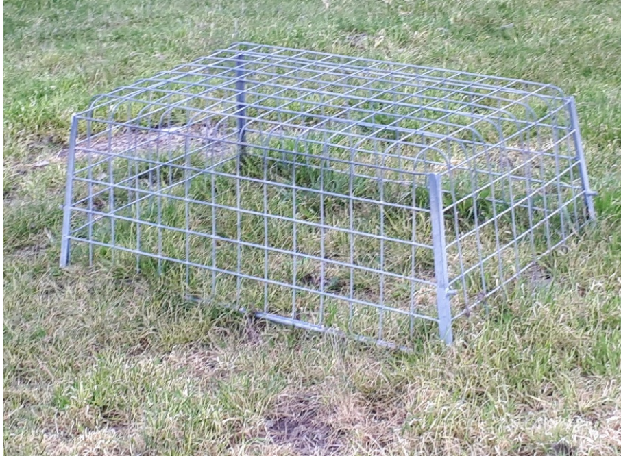
Plate 1: An example of an enclosure cage. Note the sloping sides which allow the cages to be stacked for transport and the short pins sticking out at each corner, which prevent the cages jamming together when they are stacked and being transported.
