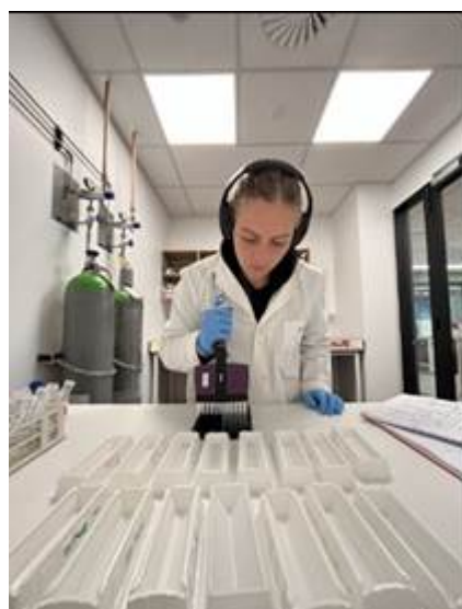
Figure 6 (right) Plating of enzyme substrates for analysis and (left) Mehlich P analysis using Murphy Riley colourimetry procedure. Bluer = more phosphorus.
